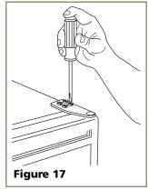
Tighten top hinge screws. Go on to 6 Prepare Power Supply.
